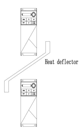
Figure 5-1-3 Multiple machines installed up and down
