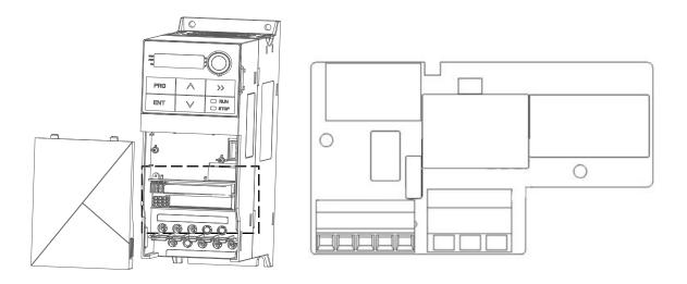
Figure 5-3-1 Expansion board diagram
