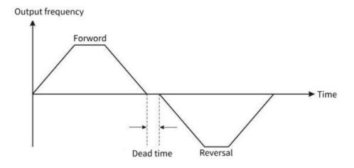
Figure 9-8-2 Reverse rotation dead zone time diagram
