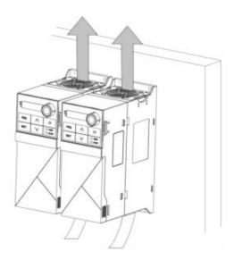
Figure 5-1-2 Multiple machines installed side by side
