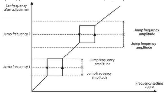
Figure 9-8-1 Jump frequency diagram
