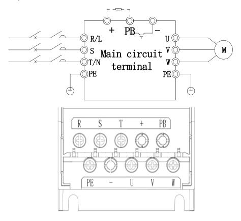
Figure 4-4-1 Main circuit terminal
