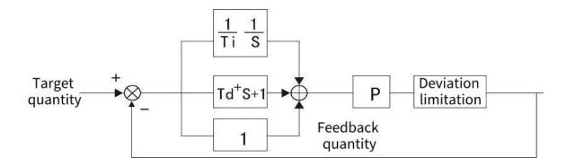
Figure 9-9-1 Process PID schematic diagram
