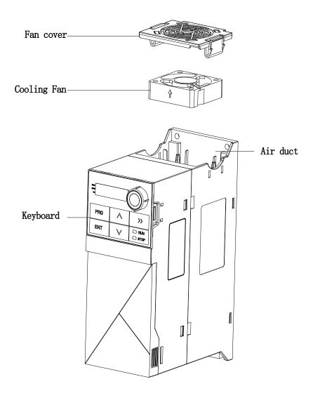
Figure 3-3-5 Detachable diagram of an independent fan
