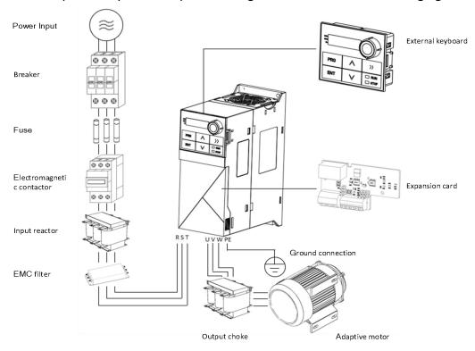
Figure 1-5-1 System construction diagram
