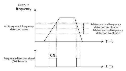
Figure 9-8-5 Schematic diagram of detection of arbitrary arrival frequency
