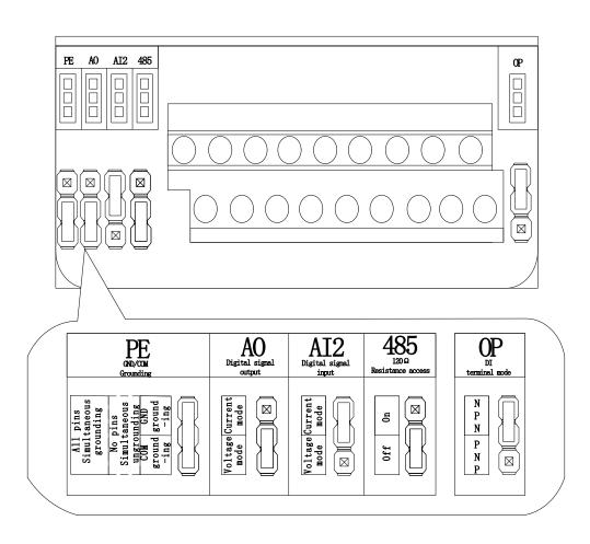
Figure 4-5-2 Jumper terminal function diagram 1
