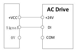
Figure 5-4-4 DI (PNP) schematic diagram
