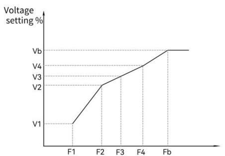
V1-V4: Percentage of voltage in the 1-4 segments Frequency Hz of multi-segment V/F
