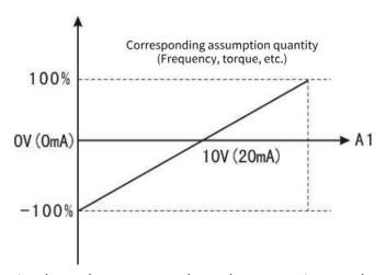
Figure 9-5-1 simulates the correspondence between given and set quantities
