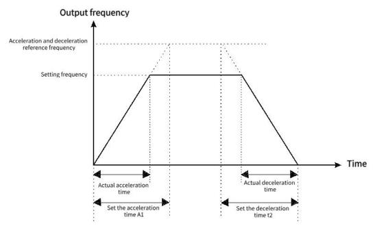
Figure 9-0-1 Acceleration and deceleration time
