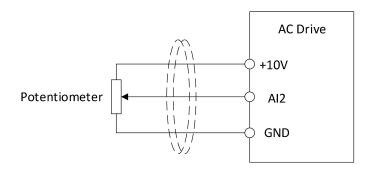
Figure 5-4-1 Voltage type wiring diagram
