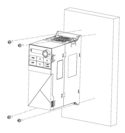
Figure 5-2-1 Screw installation diagram
