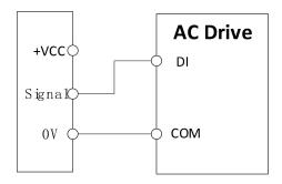
Figure 5-4-3 DI (NPN) Power supply wiring diagram
