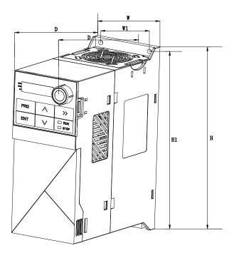
Figure 4-1-2 Dimensions V1 parameters
