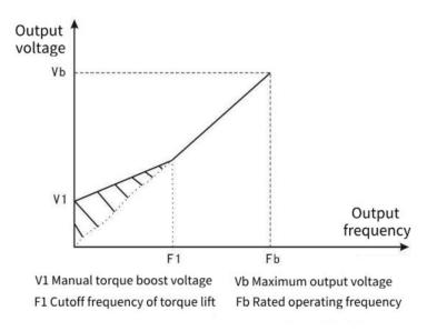
Figure 9-4-1 Manual torque raising diagram
