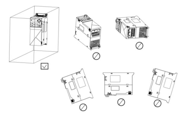
Figure 5-1-4 Installation direction diagram
