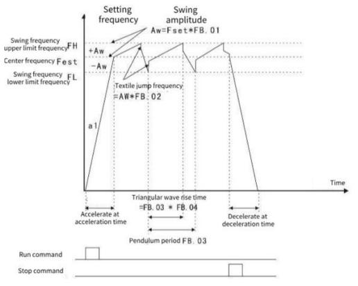
Figure 9-B-1 Schematic diagram of swing frequency operation
