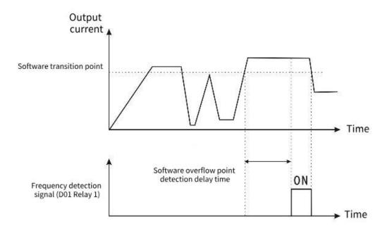
Figure 9-8-8 Schematic diagram of software overflow point detection
