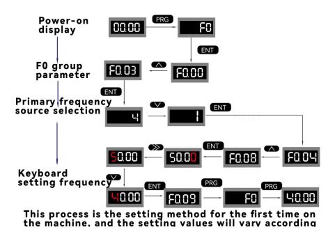
Figure 2-2-1 Rapid debugging process
