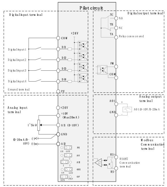
Figure 4-5-1 Control loop terminal diagram
