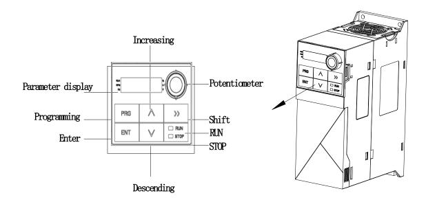
Figure 2-1-1 Operation panel diagram
