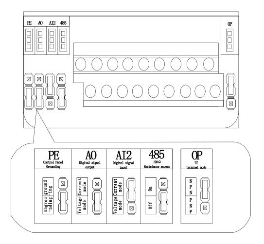
Figure 4-5-3 Jumper terminal function diagram 2
