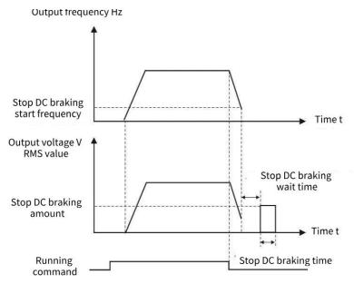
Figure 9-1-1 Shutdown DC braking diagram
