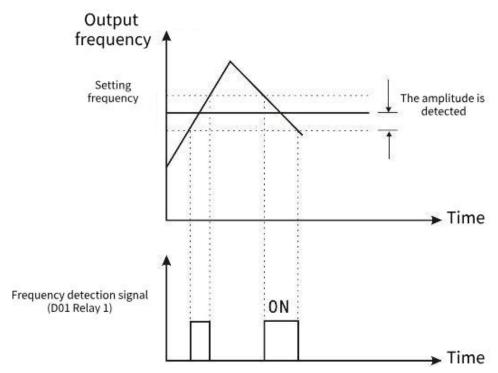
Figure 9-8-4 Schematic diagram of frequency arrival detection amplitude
