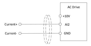
Figure 5-4-2 Current mode wiring diagram
