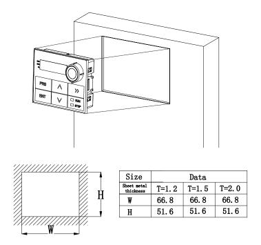
Figure 3-1-2 Panel opening dimensions diagram
