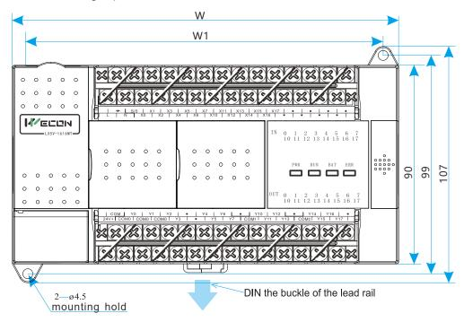
Use the M4 screw to install the PLC. The distance and the location refer to the right figure.
