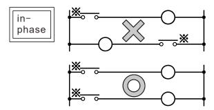
•Contactors of forward and reverse close very dangerous at the same time, like this load, except to use internal program to do interlock control, on the outside of the programmable controller must also set the interlock.
