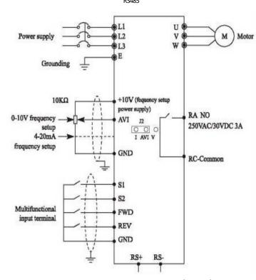
Solution Note: AVI terminals can be used to select an analog voltage input(0-10V) and analog current input (4-20mA) through the switch J2.
