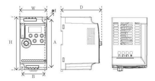
Note: Standard 35mm rail installation is supported below 5.5KW. Unit: mm
