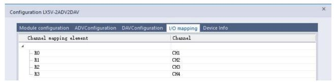
5、 After the above configuration is completed, check the program, download the configuration to PLC, and STOP→RUN configuration takes effect.
