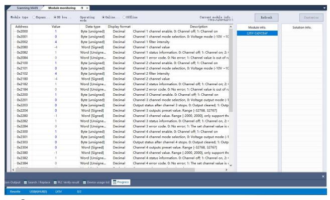
(1) ADV buffer memory (BFM): used for BD module status monitoring.
