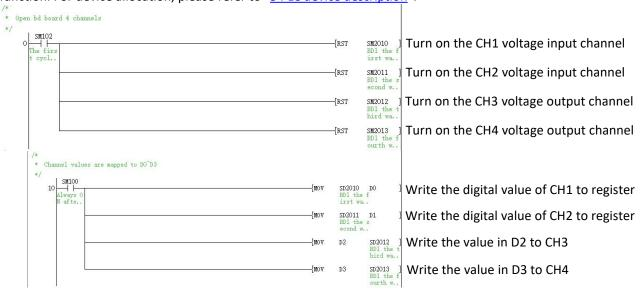
2. Programming example using "BD module configuration" function of host computer software:
