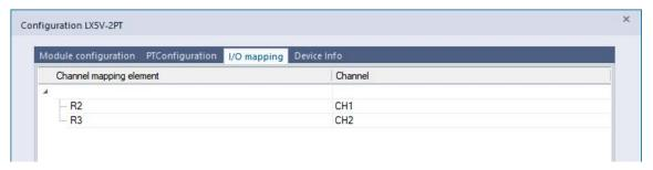
4、 After the above configuration is completed, check the program, download the configuration to PLC, and STOP→RUN configuration takes effect.
