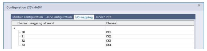
4、 After the above configuration is completed, check the program, download the configuration to PLC, and STOP→RUN configuration takes effect.
