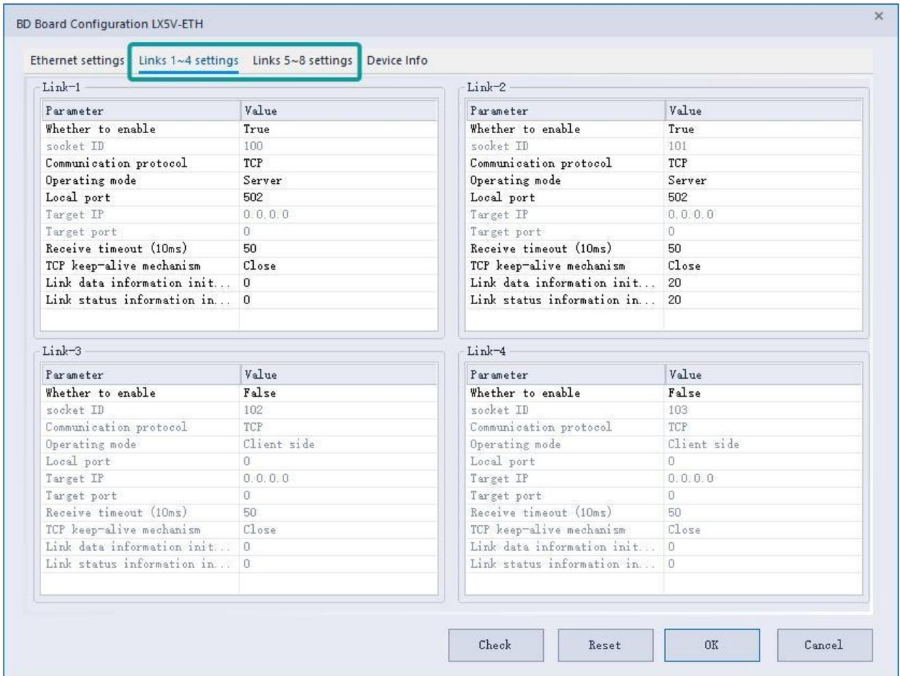
**Note:** One LX5V-ETH-BD supports up to 8 Ethernet links, each of which can be individually configured to enable.
