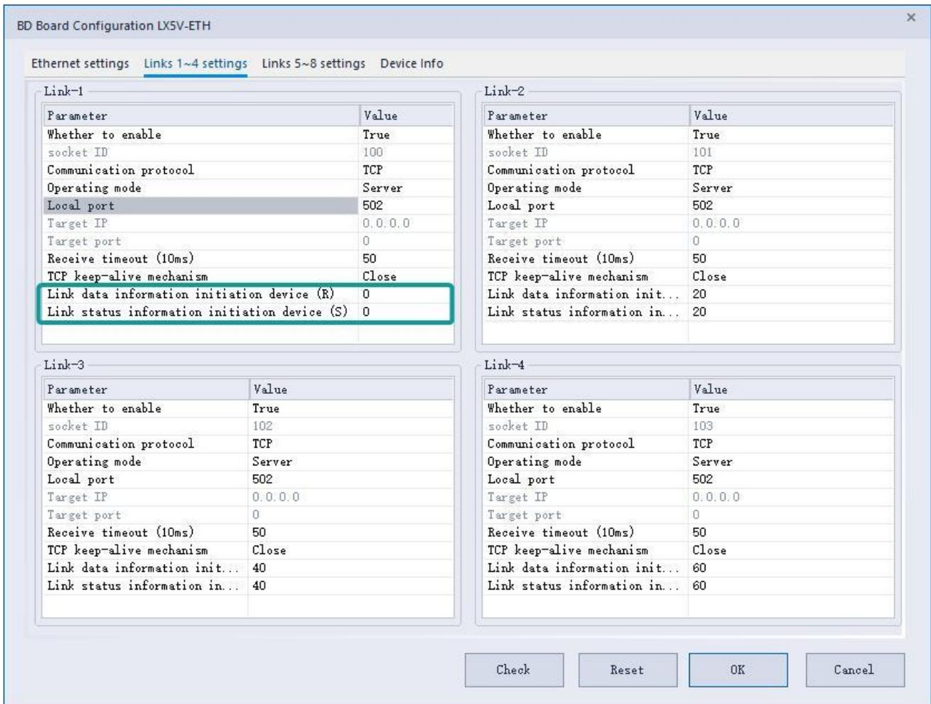
**Note:** The server needs to configure "link data information initial device" and "link status information initial device", and the settings of each link should not overlap.
