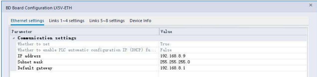
**Note:** The IP address should be configured in the same network segment as the IP address of the master station. For example, if the IP address of the master station is 192.168.8.8 and the subnet mask is 255.255.255.0, the IP address of the BD module should be configured as 192.168.8.xx (the value of xx is 1to255. Do not duplicate other IP addresses on the same network segment).
